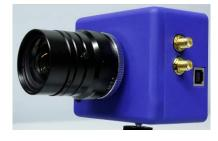
5 –reconfigurable user-friendly compact camera module for 2D/3D acquisitions of pictures and movies by any (linear array or imager, iTOF or dTOF based) MiSPiA CMOS SPAD imagers, to be remotely controlled by a remote pc through USB 2.0 link and a graphical user interface. All smart processing can be performed on-board thanks to a powerful FPGA and SRAM, able to store high-throughput streams of data. The software
