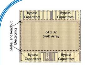
3 – a set of 3D ranging **imagers for and photon-counting** with among the best cutting-edge performance among SPAD imagers for 3D "indirect TOF", based on smartpixels with 30 $\mu$ m SPADs and digital counters for phaseresolved detection of either pulsed-light (PL) or continuous-wave (CW) actively illuminate scenes: linear arrays or 64x32 imagers acquiring 2D images at 100,000fps and 3D maps movies at 33,000fps, with 9bit photon-counting dynamics. Beyond 3D ranging, these
