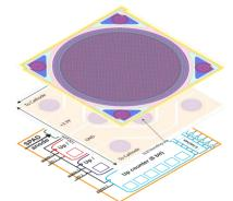
performance all-silicon CMOS SPAD imagers in compact onechip solution. The BackSPAD technology instead allow to exploit the best detection performance out of the SOI SPAD together with the best counting and timing performance out of the CMOS electronics. Further exploitation of the BackSPAD technology is to bridge the gap among Silicon SPADs and III-V semiconductor-based devices, to provide single-photon sensitivity to advanced imaging in the near-
