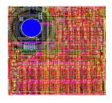
2 - a set of 3D ranging **imagers for photon-timing** with best-detection performance so far reported, based on smart-pixels with 30µm SPADs and in-pixel time-to-digital converters (TDCs) for direct TOF measurement of individual single photons: both linear arrays and 32x32 imagers, acquiring 2D images and 3D movies at 100,000 frames/s fps with 5cm single-shot
